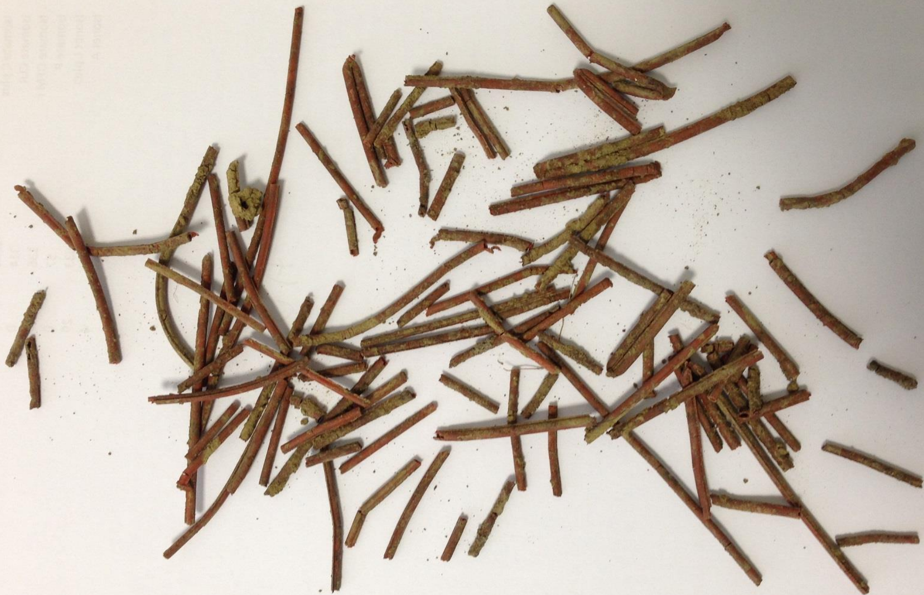
Shin-Etsu biodegradable dispensers after 7 months in the soil
