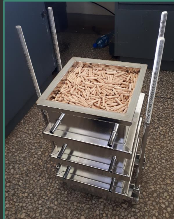
Fermenter filled with the wooden dowels
